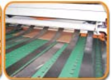
Vacuum head after knife on Fosber sheeter
