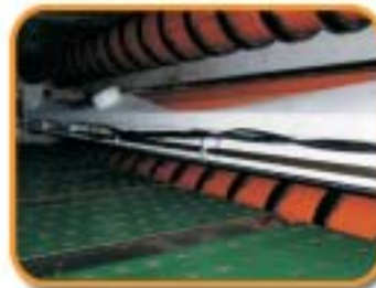
Vacuum head after knife on Fosber sheeter
