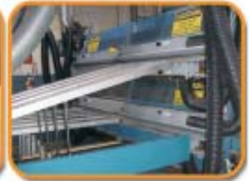
Cleaning two webs after slitting and web split
