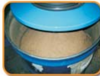
3 week's dust gathered after knife on corrugator
